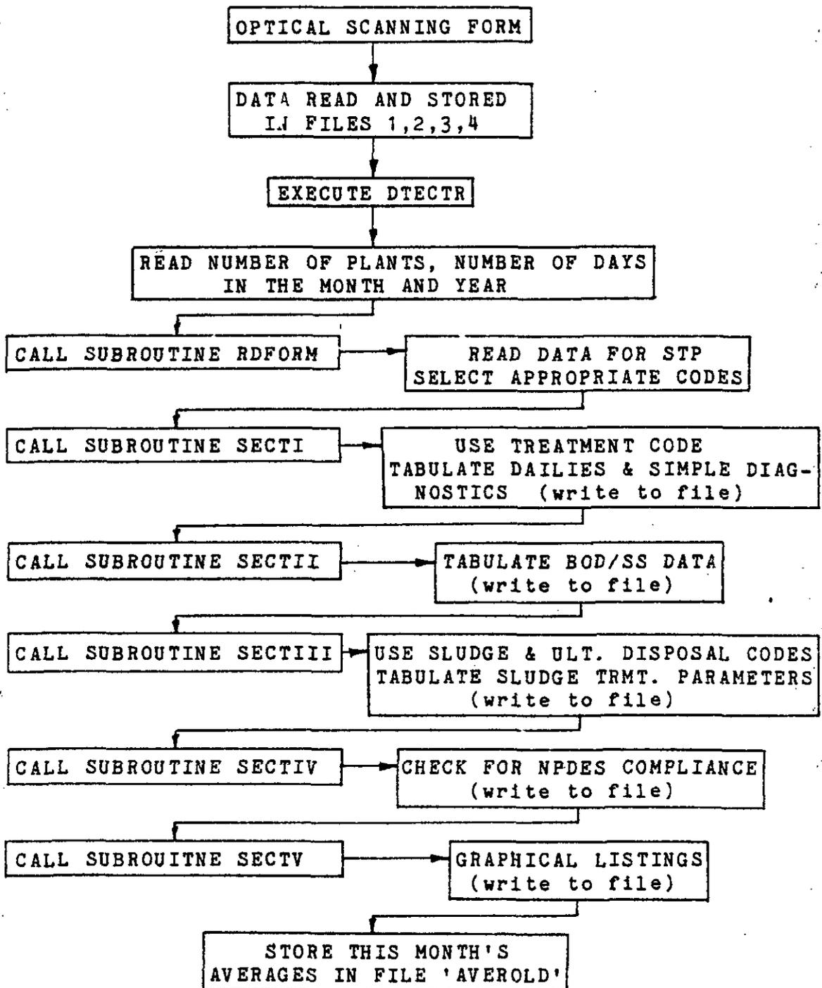
Figure 2. Idealized DTECTR Flow Diagram.
